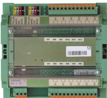
The ZENIX DI12 is a field device with 12 potential free digital inputs. It can be used to connect additional alarm inputs from the fire detection panel (matrix). It can also be used to connect field inputs such as end switches of mechanical dampers, for example.
