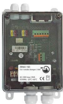
The ZENIX 1SD field device is used to monitor and control 1 motorized smoke control damper with 230 V actuator. No configuration is required as it has a predefined device address.
