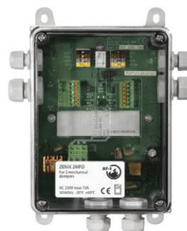
The ZENIX 2MFD field device is used to monitor up to 2 mechanical (fusible link) dampers. No configuration is required as it has a predefined device address.
