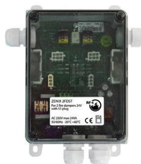
The ZENIX 2FDST field device is used to monitor and control up to 2 motorized fire dampers with 24 V actuator with ST-connection plugs. No configuration is required as it has a predefined device address.
