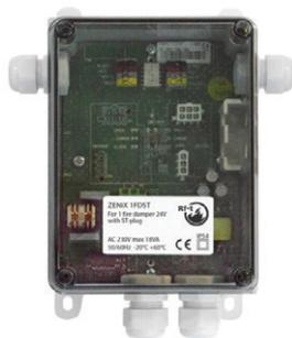
The ZENIX 1FDST field device is used to monitor and control 1 motorized fire damper with 24 V actuator with ST-connection plugs. No configuration is required as it has a predefined device address.
