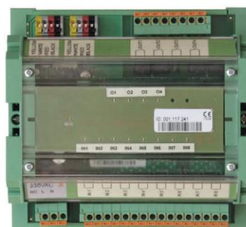
The ZENIX DI8DO4 is a field device with 8 potential free digital inputs and 4 digital relay outputs. It can be used to connect additional alarm inputs from the fire alarm panel (matrix), for example. Relay outputs can be programmed, and safe states be defined as required.
