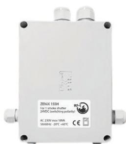
The ZENIX 1SSH field device is used to monitor and control 1 motorized smoke control shutter 24 V. The shutter's actuator is triggered via 2 wires: switching the polarity allows the blade to move in the other direction. The ZENIX 1SSH has 4 digital inputs and 2 relay outputs.
